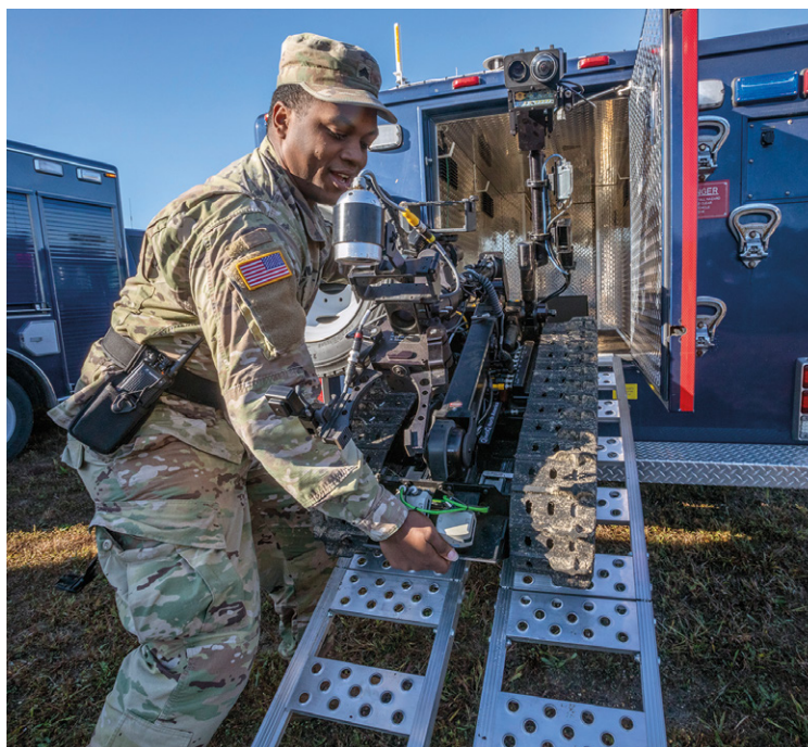
U.S. Army Sgt. Quran T. Williams unloads a Talon IV robot. The robot is used for reconnaissance and detection in chemical, biological, radiological, and nuclear environments. (New Jersey National Guard photo by Mark C. Olsen via flickrr, license CC BY 2.0.)
