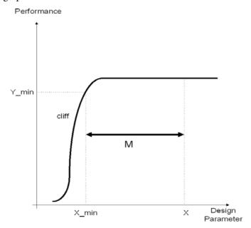
Current U.S. warheads have rather tight (small) performance margins: they were designed in the 1980s, where miniaturization of the warhead and maximization of its yield to weight ratio was emphasized; they operated close to the 'performance cliff', but extensive test series made sure that the weapon always performed above the critical threshold throughout its life-cycle.
